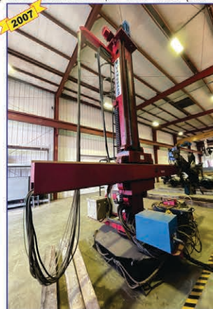
Clad Unit #5: Vanguard LHZ34 Cladding Machine with Arc Specialties Hot One Solid State Hotwire Power Supply Esab MTS-3500i MIG Welder, Note: (2) rotary tables avail.
